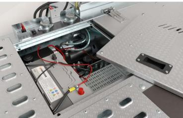
Power and systems enclosure allows easy access to battery, hydraulic pump and optional control units.
