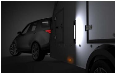
Super bright side mounted LED reverse lights provide valuable extra visibility for close the trailer interior. Switched separately.
