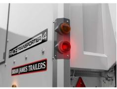
• High quality lighting system - automotive specification lamps stylishly mounted. Front and side marker lamps are LED technology as standard.
