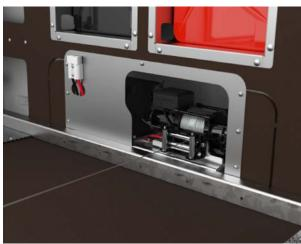
• Electric winch, 12V with remote control lead. 4,500 lbs capacity, roller fairlead, wire cable and snap hook, plus on-board battery power. Separate mains battery charger also included.
