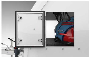
• Front access hatches are convenient for reaching inside during vehicle strapping.
