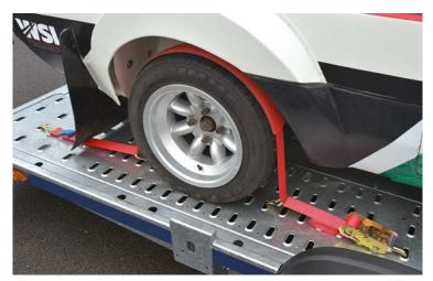
**O Tie-down wheel 'sleeve' straps** Approved by car manufacturers and race teams alike, these new straps hold the vehicle safely and securely without straining suspension geometry. Easy to fit, with multiple built-in tie-down points.
