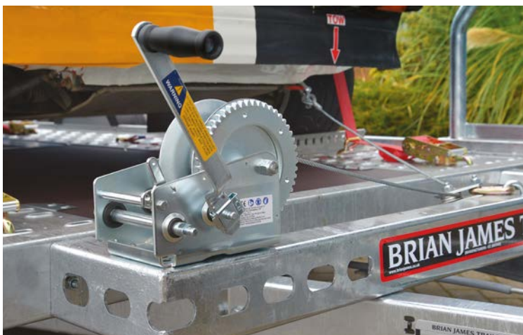
○ Manual winch + 3 point adjustable pull positions.
