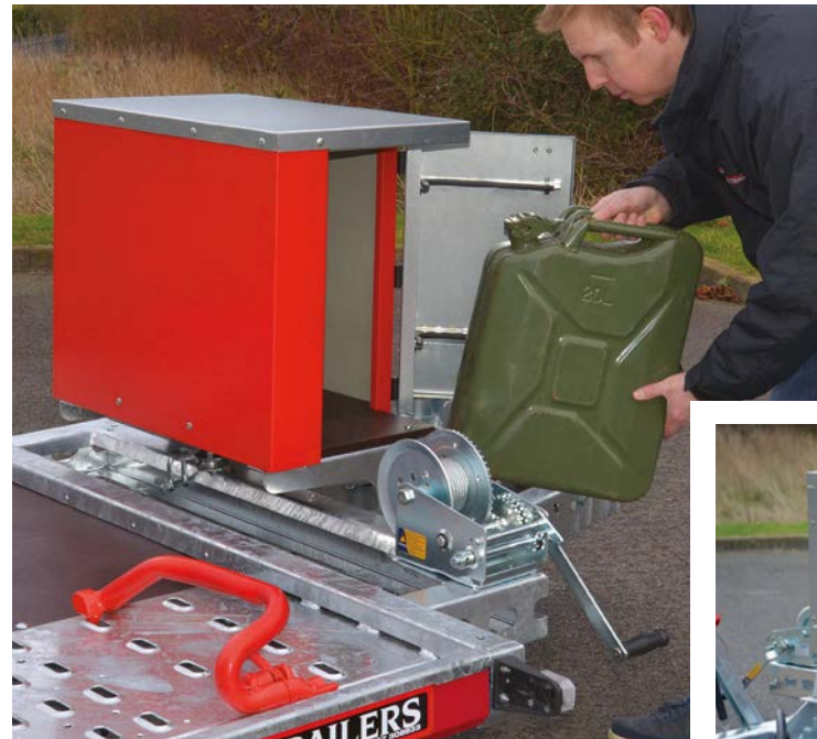
○ Fuel can storage Designed to carry either 1, 2 or 3 x 20ltr Jerry cans. Lockable, twin opening doors. A Transporters are available in Sargasso blue, Poppy red, Arcelor anthracite or Jet black body colour trim and the fuel storage locker can be colour matched to the trailer body.
