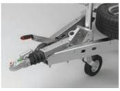
• Level ride, matched coupling Models with larger wheels are fitted with a lowered draw bar, ensuring that the tow ball is matched to the optimum height for level towing.
